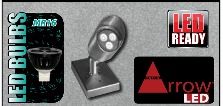
FL-LED-MR16 4 WATT UNIVERSAL PLUG & PLAY MR16 BI-PIN STYLE LED 2 POPULAR BEAM SPREADS: 35° (BAB) AND 12° (ESX) 50,000 HOURS AVERAGE RATING WARM WHITE (2900K) HIGH POWER/HIGH LUMEN OUTPUT OPERATES ON 12V AC/DC SYSTEMS (OPTIMUM RANGE 10V-15V) MUST USE WITH MAGNETIC TRANSFORMERS ONLY
