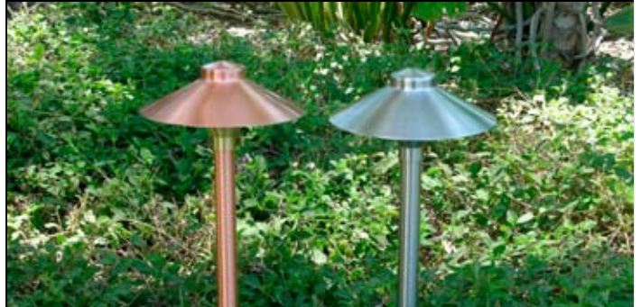
RXA-01-COP/RXA-01-SS SPUN COPPER OR STAINLESS STEEL 6" CHINA HAT AREA LIGHT CAST BRASS OR CAST STAINLESS STEEL ADJUSTABLE HUB STANDARD 6" X 15" 20W T-3 S.C. HALOGEN
